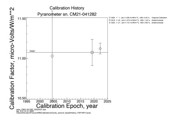
Calibration history for pyranometer CM21-041282. The solid horizontal line represents the mean value. The symbols and their error bars represent the mean and U95 of each calibration event. The column on the right presents numerical values for each calibration event and a brief description of the calibration method used.
