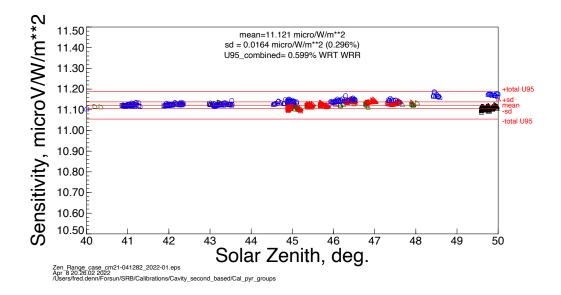
Calibration coefficients for several days. Each symbol represents an individual calibration value. The mean of these values will be taken to be the final calibration value. The overall U95 uncertainty is also displayed here.
