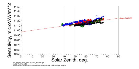
Calibration coefficients for, all zenith angles, several days. This displays the solar zenith angle dependance of the calibration values.
