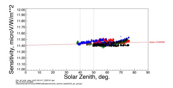
Calibration coefficients for several days. This displays the solar zenith angle dependance of the calibration values. Calibration coefficients for several days. Each symbol represents an individual calibration value.
