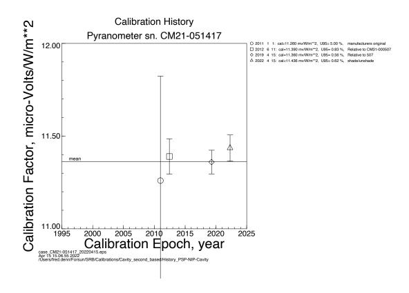
Calibration history for pyranometer CM21-051417. The solid horizontal line represents the mean value. The symbols and their error bars represent the mean and U95 of each calibration event. The column on the right presents numerical values for each calibration event and a brief description of the calibration method used.
