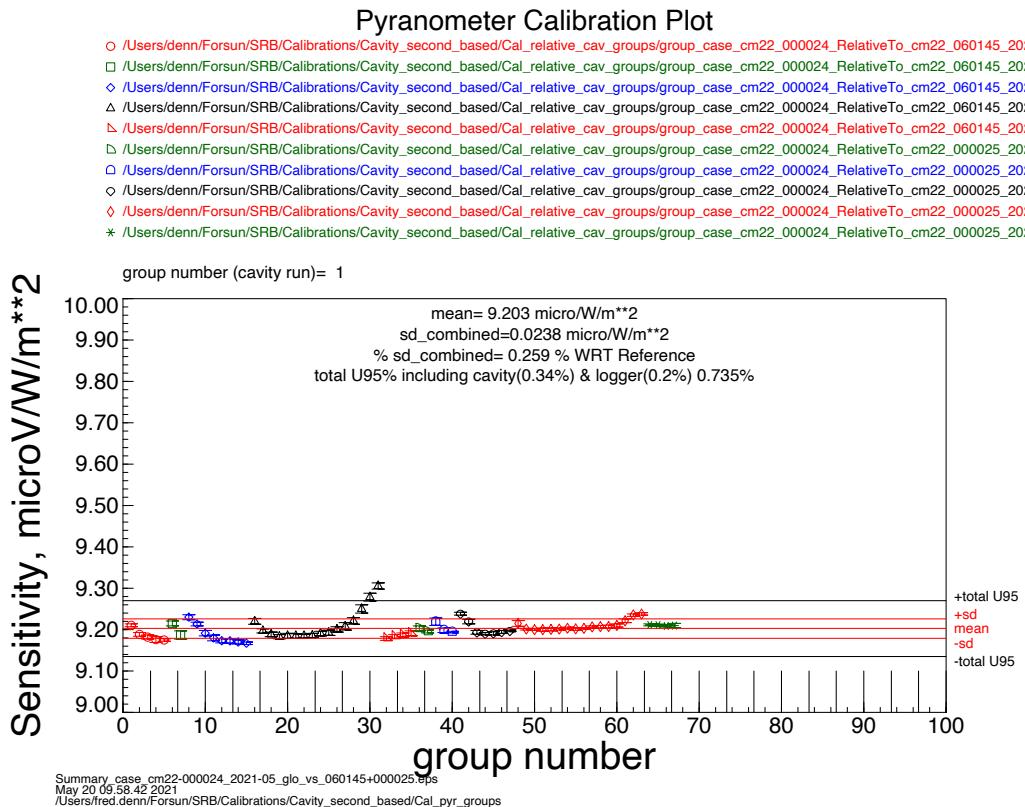
Calibration coefficients for several days. Each symbol represents a cavity run which is approximately 25 minutes. These data are combined to get a final calibration coefficient for the entire, multi-day, calibration session. The final calibration value is the mean of the calibrations relative to CM22-060145 and CM22-000025.
