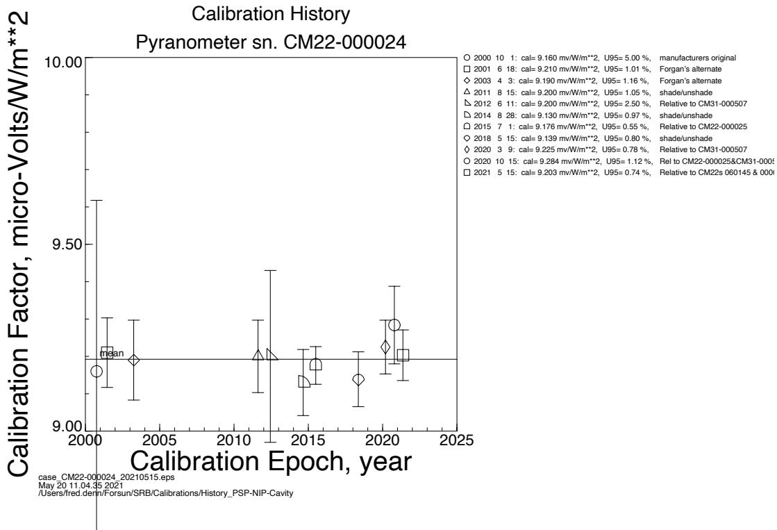
Calibration history for pyranometer CM22-000024. The solid horizontal line represents the mean value. The symbols and their error bars represent the mean and U95 of each calibration event. The column on the right presents numerical values for each calibration event and a brief description of the calibration method used.
