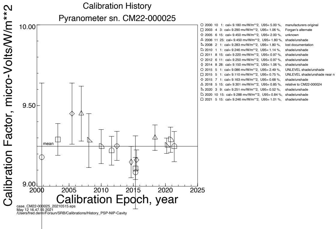
Calibration history for pyranometer CM22-000025. The solid horizontal line represents the mean value. The symbols and their error bars represent the mean and U95 of each calibration event. The column on the right presents numerical values for each calibration event and a brief description of the calibration method used.
