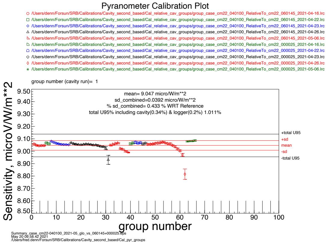
Relative calibration coefficients for several days. Each symbol represents a cavity run which is approximately 25 minutes. These data are combined to get a final calibration coefficient for the entire, multi-day, calibration session. Data are for CM22-040100 relative to pyranometers CM22-060145, and CM22-000025, which were calibrated with the shade/unshade method.
