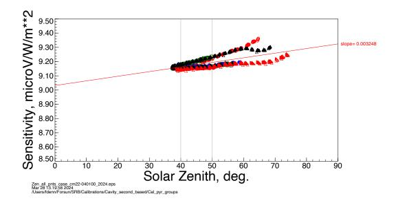
Calibration coefficients for, all zenith angles, several days. This displays the solar zenith angle dependance of the calibration values.
