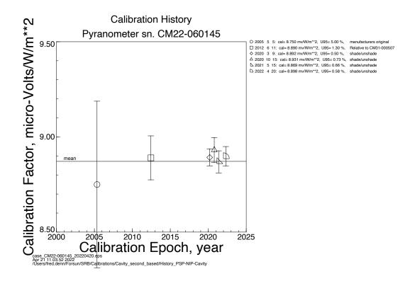
Calibration history for pyranometer CM22-060145. The solid horizontal line represents the mean value. The symbols and their error bars represent the mean and U95 of each calibration event. The column on the right presents numerical values for each calibration event and a brief description of the calibration method used.
