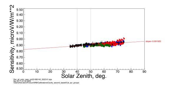
Calibration coefficients for, all zenith angles, several days. Each symbol represents a cavity run which is approximately 25 minutes. This displays the solar zenith angle dependance of the calibration values.
