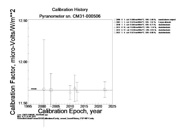
Calibration history for pyranometer CM31-000506. The solid horizontal line represents the mean value. The symbols and their error bars represent the mean and U95 of each calibration event. The column on the right presents numerical values for each calibration event and a brief description of the calibration method used.
