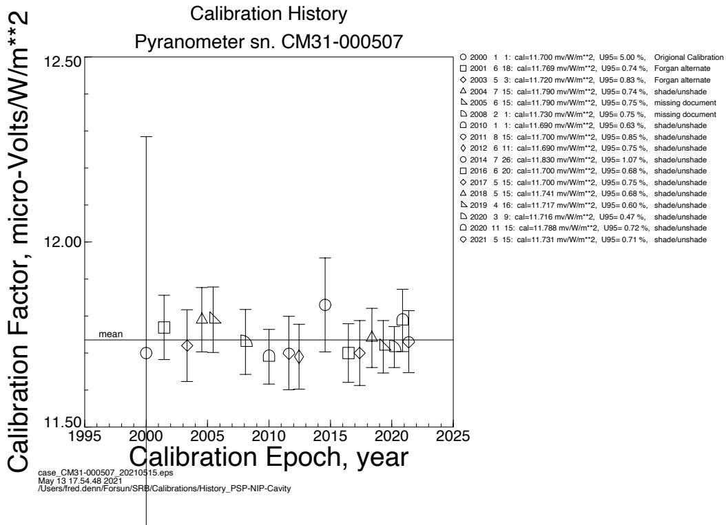
Calibration history for pyranometer CM31-000507. The solid horizontal line represents the mean value. The symbols and their error bars represent the mean and U95 of each calibration event. The column on the right presents numerical values for each calibration event and a brief description of the calibration method used.
