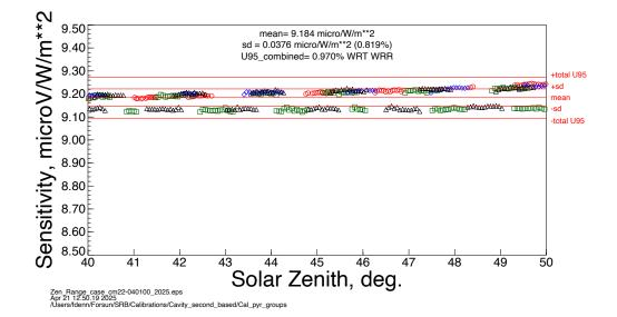
Calibration coefficients for several days. Each symbol represents an individual calibration value. The mean of these values will be taken to be the final calibration value. The overall U95 uncertainty is also displayed here. Data is limited to solar zenith angles 40° through 50°.
