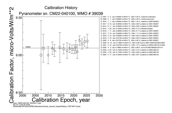
Calibration history for pyranometer CM22-040100. The solid horizontal line represents the mean value. The symbols and their error bars represent the mean and U95 of each calibration event. The column on the right presents numerical values for each calibration event and a brief description of the calibration method used.
