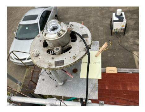
Photo of pyranometer CM22-040100 mounted on a fixed stand Note the position. North is to the right. This pyranometer has been calibrated and used in the same position. Although it is hard to see here there is a small hole in the sensor just inside the domes radially in form the mounting screw near the level. We have not seen a similar hole on any other pyranometers.
