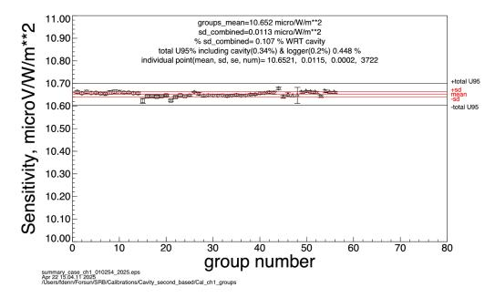
Calibration coefficients for several days. Each symbol represents a cavity run which is approximately 25 minutes. These data are combined to get a final calibration coefficient for the entire, multi-day, calibration session.
