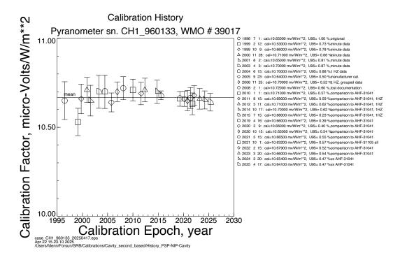
Calibration history for pyrheliometer CH1-960133. The solid horizontal line represents the mean value. The symbols and their error bars represent the mean and U95 of each calibration event. The column on the right presents numerical values for each calibration event and a brief description of the calibration method used.
