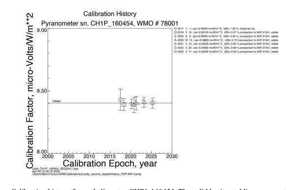
Calibration history for pyrheliometer CHP1-160454. The solid horizontal line represents the mean value. The symbols and their error bars represent the mean and U95 of each calibration event. The column on the right presents numerical values for each calibration event and a brief description of the calibration method used.
