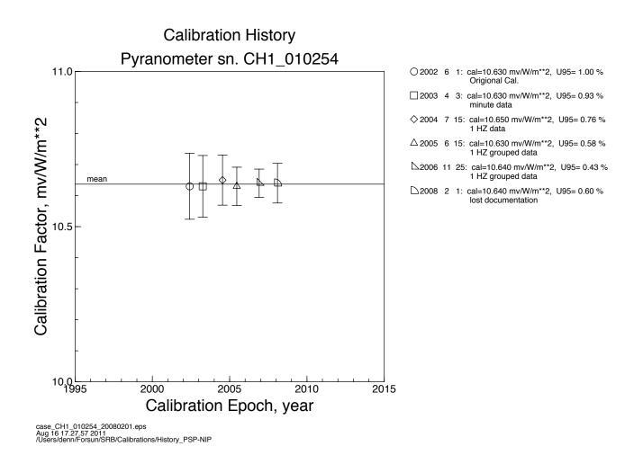
Figure 5. Calibration history for pyrheliometer CH1-010254 is presented. The solid horizontal line represents the mean value. The symbols and their error bars represent the mean and U95 of each calibration event. The column on the right presents numerical values for each calibration event and a brief description of the calibration method used.
