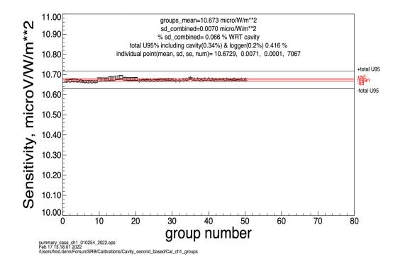
Calibration coefficients for several days. Each symbol represents a cavity run which is approximately 25 minutes. These data are combined to get a final calibration coefficient for the entire, multi-day, calibration session.
