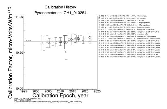
Calibration history for pyrheliometer CH1-010254. The solid horizontal line represents the mean value. The symbols and their error bars represent the mean and U95 of each calibration event. The column on the right presents numerical values for each calibration event and a brief description of the calibration method used.
