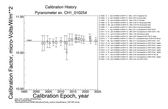
Calibration history for pyrheliometer CH1-010254. The solid horizontal line represents the mean value. The symbols and their error bars represent the mean and U95 of each calibration event. The column on the right presents numerical values for each calibration event and a brief description of the calibration method used.
