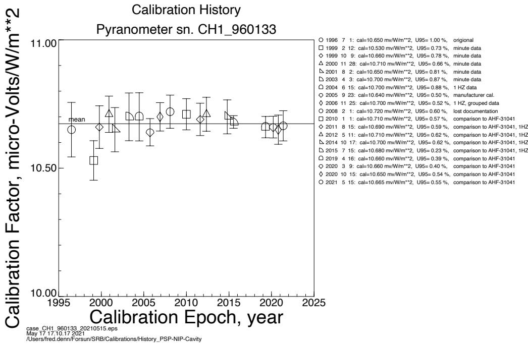
Calibration history for pyrheliometer CH1-960133. The solid horizontal line represents the mean value. The symbols and their error bars represent the mean and U95 of each calibration event. The column on the right presents numerical values for each calibration event and a brief description of the calibration method used.
