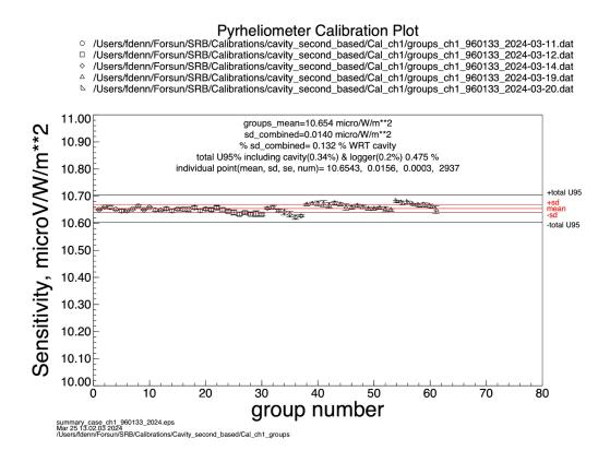
Calibration coefficients for several days. Each symbol represents a cavity run which is approximately 25 minutes. These data are combined to get a final calibration coefficient for the entire, multi-day, calibration session.
