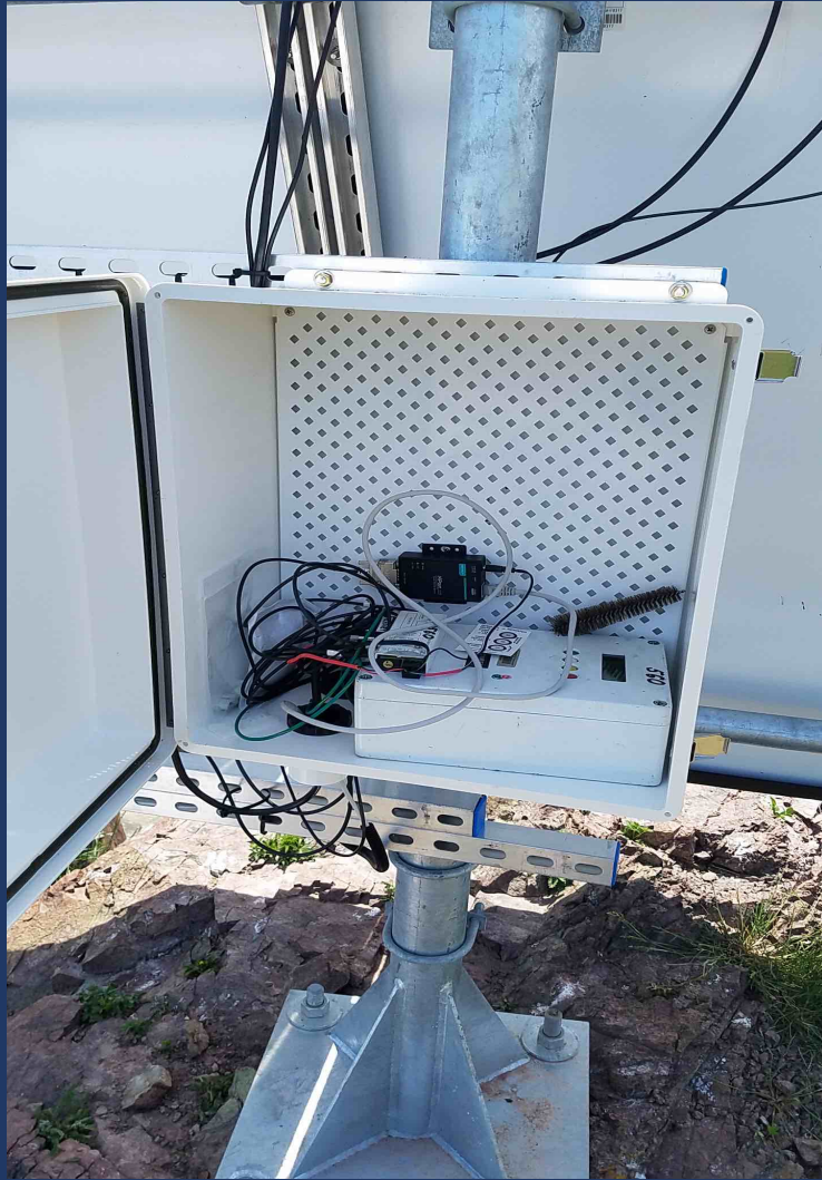
AERONET control box with MOXA serial over IP connection
