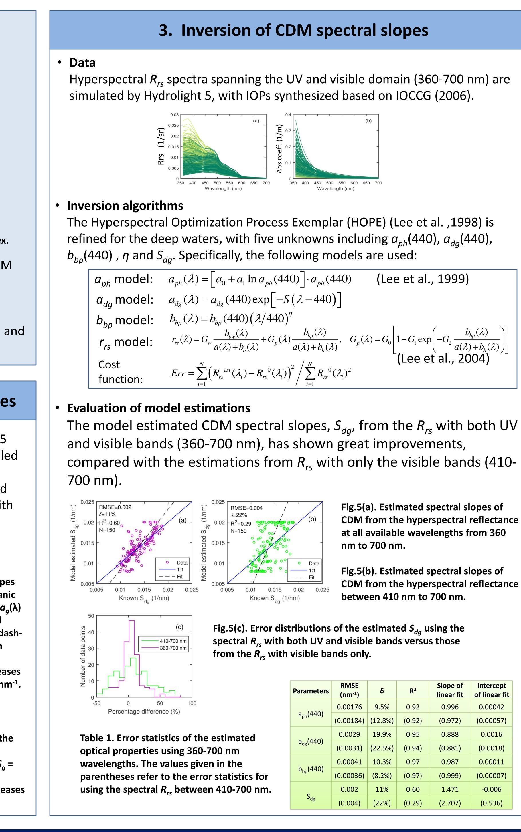
$$G_{p}(\lambda) = G_{0} \left[ 1 - G_{1} \exp \left( -G_{2} \frac{b_{bp}(\lambda)}{a(\lambda) + b_{b}(\lambda)} \right) \right]$$
