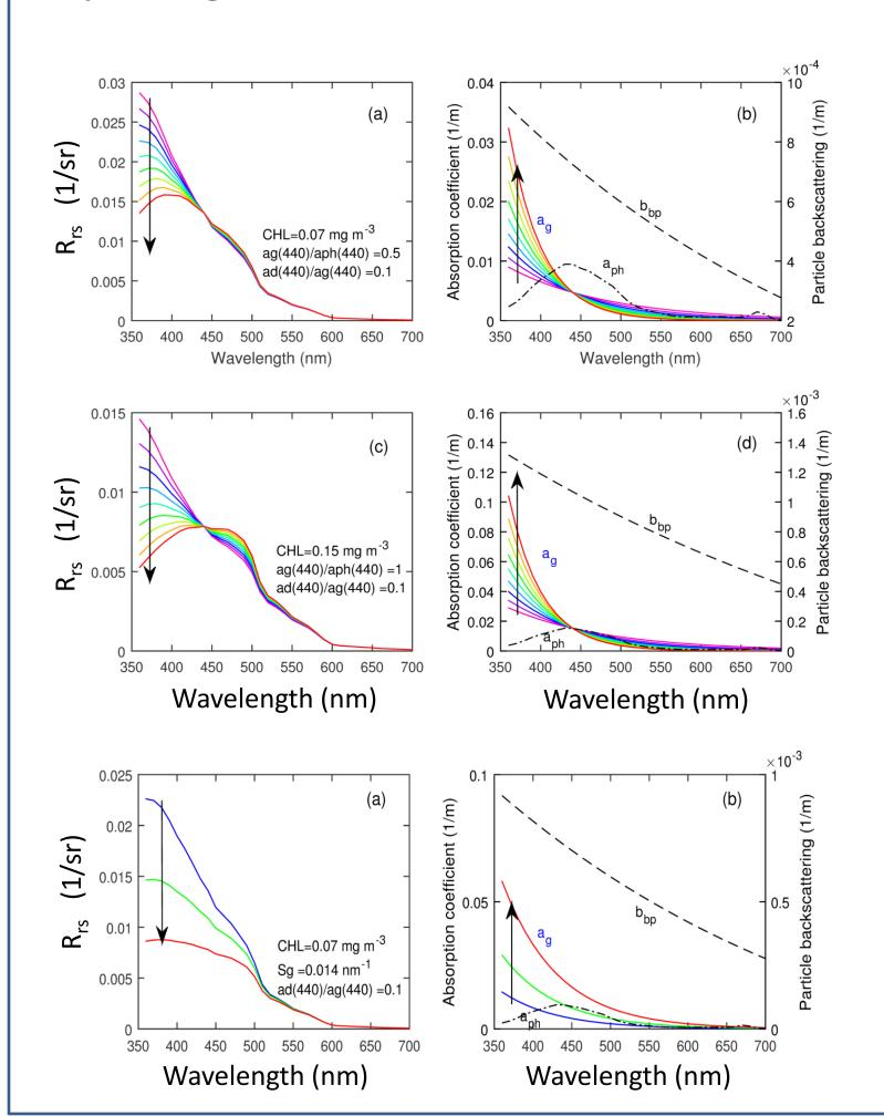
Fig.2 Variation of R<sub>rs</sub> spectra shapes with different spectral slopes of CDOM in two oceanic waters. The spectral  $a_a(\lambda)$ is denoted in colored lines,  $a_{ph}(\lambda)$  in black dashdot line, and  $b_{bp}(\lambda)$  in black dash line. The CDOM slope,  $S_a$  increases from 0.008 to 0.024 nm<sup>-1</sup>.
