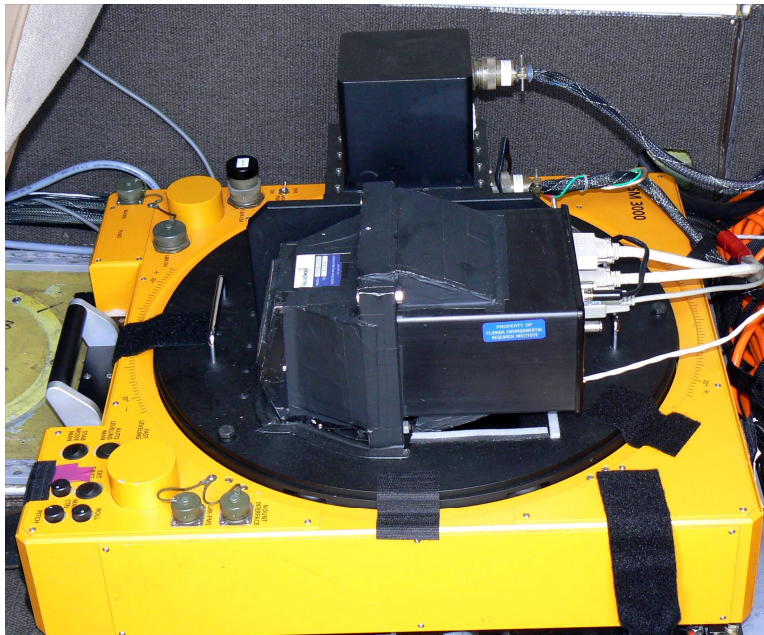
Fig. 3. The Spectroscopic Aerial Mapper with On-board Navigation (SAMSON). The hyperspectral imager is black object in the foreground. The black box at the top of the image is the integrated inertial navigation system which sits atop a high resolution framing camera. The yellow frame is the motion compensation mounting system.
