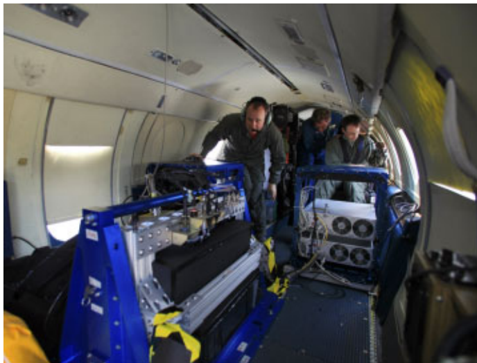
Figure 5-2. Tom Delker (left) and Jeremy Craner (right) from Ball Aerospace, with NASA Langley's Les Kagey (center), installing the GEO-TASO instrument on the NASA Falcon in 2013. GEO-TASO is a test bed for the TEMPO instrument. (Image Credit: NASA/David C. Bowman)
