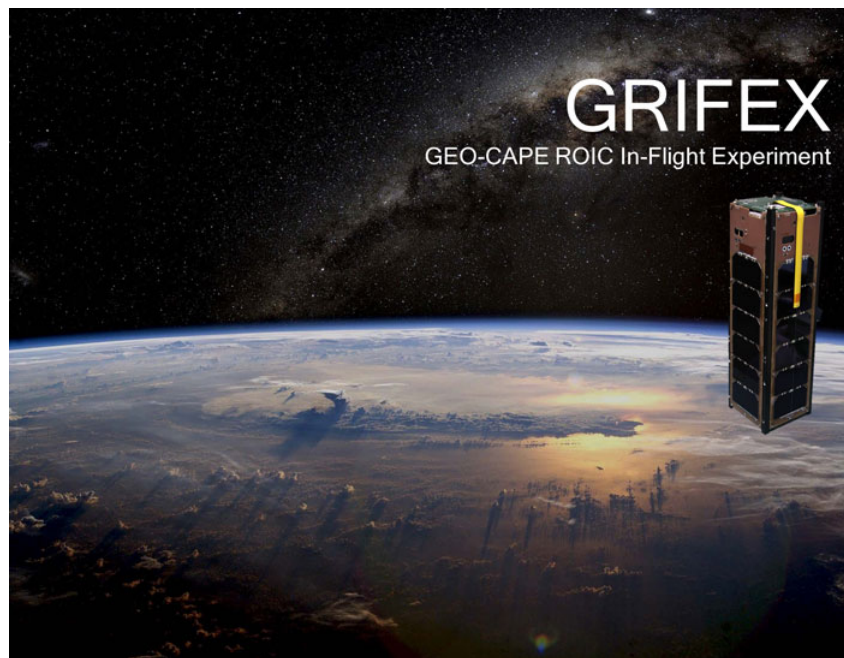
Figure 5-3. A 3-unit CubeSat launched in 2015 to validate the ROIC technology (Image Credit: NASA JPL and U. Michigan).
