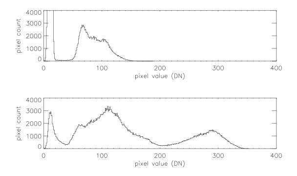
**Figure 3.** Histograms of raw pixel counts for the two subsampled regions. *Top*: for the Moon image of Figure 2(a), *Bottom*: for the Earth scene of Figure 2(b). Both histograms were generated using full-disk image data, uncorrected for oversampling.
