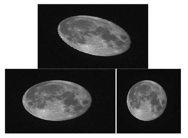
**Figure 4.** Steps in GOES-12 lunar image processing. *Top:* subsample of the full-disk image, uncorrected for oversampling. *Lower left:* with scan line offset correction to remove the apparent motion of the Moon across the FOR. *Lower right:* with oversampling correction based on an elliptical limb fit.
