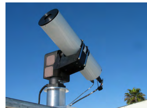
Figure 5. OSPREy radiance radiometer mounted on the pointing device and tracking the Sun.
