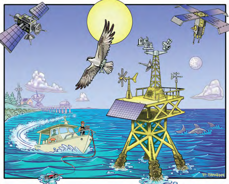
Figure 1. Deployment example for an OSPREy system in support of ocean color research: an OSPREy Operational System (Fig. 7.4), consisting of two EPIC dyads, is mounted on top of an offshore tower. Also shown are solar panels and a wind generator for providing power; the ocean color satellite to be validated; a telecommunications satellite for data telemetry; a shore-based calibration and logistical support facility; and regular quality control visits using a small boat. The latter includes the sampling of in-water optical profiles with the C-PHIRE System shown in Fig. 8.
