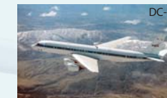
DC-8 Role: Tropospheric in situ sampling, vertical profiles, remote sensing using radars, lidars & radiometers Altitude: 41,000 ft Payload: 30,000 lbs Range: 5,400 Nmi
