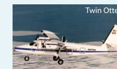
Twin Otter Role: Low-altitude remote sensing and in situ sampling Altitude: 25,000 ft Payload: 5,000 lbs Range: 500 Nmi
