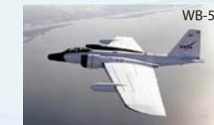
WB-57 Role: Remote sensing, Upper Tropospheric and Stratospheric in situ sampling, vertical profiling Altitude: 60,000 ft + Payload: 7,500 lbs + Range: 2,500 Nmi
