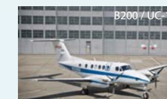
B200 / UC-12 Role: Mid-altitude remote sensing and in situ sampling Altitude: 35,000 ft Payload: 4,100 lbs Range: 1,250 Nmi
