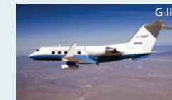
G-III Role: UAV/SAR and mid-altitude remote sensing Altitude: 45,000 ft Payload: 2,610 lbs Range: 3,400 Nmi
