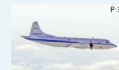
P-3 Role: Remote sensing, Laser profiling, Tropospheric in situ sampling Altitude: 30,000 ft Payload: 14,700 lbs Range: 3,900 Nmi
