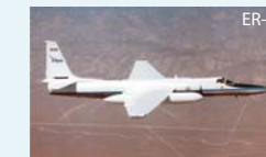
ER-2 Role: Remote sensing, Upper Tropospheric and Stratospheric in situ sampling Altitude: 70,000 ft Payload: 2,900 lbs Range: 5,000 + Nmi
