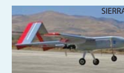
SIERRA Role: Low altitude remote sensing and in situ sampling Altitude: 12,000 ft Payload: 100 lbs Range: 550 Nmi
