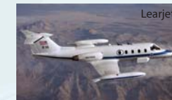
Learjet Role: Remote sensing, Upper Tropospheric and Stratospheric in situ sampling Altitude: 45,000 ft Payload: 3,200 lbs Range: 1,200 Nmi
