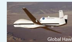
Global Hawk Role: Long duration high-altitude remote sensing; upper Tropospheric and Stratospheric in situ sampling; UAV/SAR Altitude: 65,000 ft Payload: 1,500 lbs Range: 11,000 Nmi
