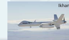
Ikhana Role: Long duration mid-altitude remote sensing and in situ sampling; real-time disaster response imaging Altitude: 52,000 ft Payload: 3,000 lbs Range: 3,500 Nmi
