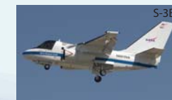
S-3B Role: Remote sensing, Upper Tropospheric and Stratospheric in situ sampling Altitude: 40,000 ft Payload: 12,000 lbs Range: 2,300 Nmi
